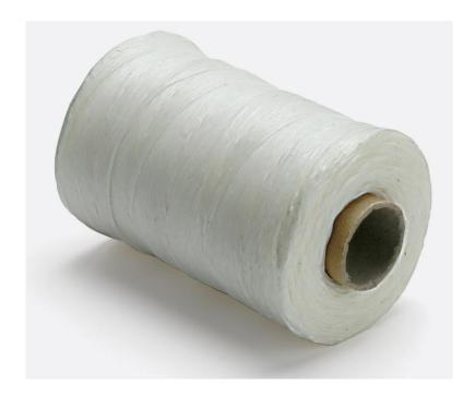
Nylon lacing cord formed as a slightly rounded mass of continuous filaments which when applied to harnesses, flattens, forms a tight knot, and will not penetrate insulations. Cord is waxed to provide excellent non-slip knots.
