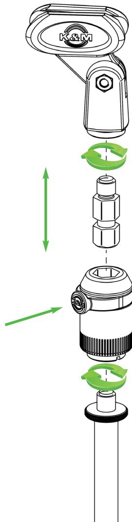
To remove the threaded bolt or to change the equipment, press the K&M logo on the grey locking ring and remove the threaded bolt upwards from the Quick-Release adapter.
