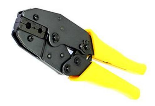
Ratchet Crimp Tool complete with die set for terminating COAX 75 ohm BNC FA size connectors requiring 1.72/1.73 Hex centre pin crimp to Canford group X broadcast cables. Die set has the following cavities:
